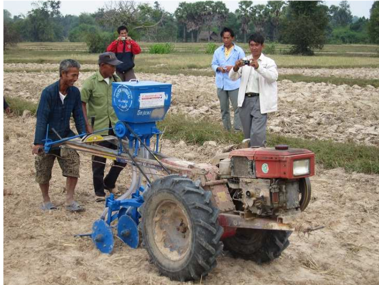
Figure 2: The Thai-built, disc-based direct seeder used in the farmer demonstration trials in western Savannakhet
