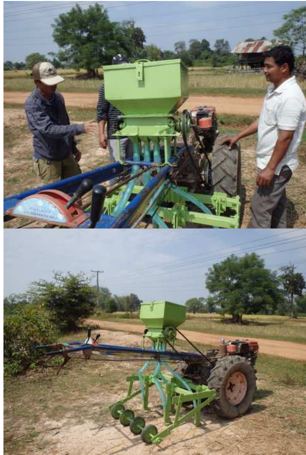
Figure 4: The modified, tine-based Thai seeder with dual seed and fertiliser box trialled by farmers in Savannakhet in wet season 2014
