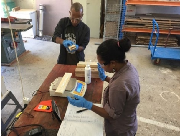
Figure 3. PNG researchers Elaine Galore of TFTC and Kilva Lancelot of PNGFRI are preparing samples for testing glue bond strength of PNG timbers (Photo credit: Benoit Belleville).
