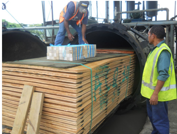
Figure 2. Bundles of wood specimens placed on top of plywood before pushing into a cylinder for treatment at PNG Forest Products PTY LTD (Photo credit: Benson Gusamo).
