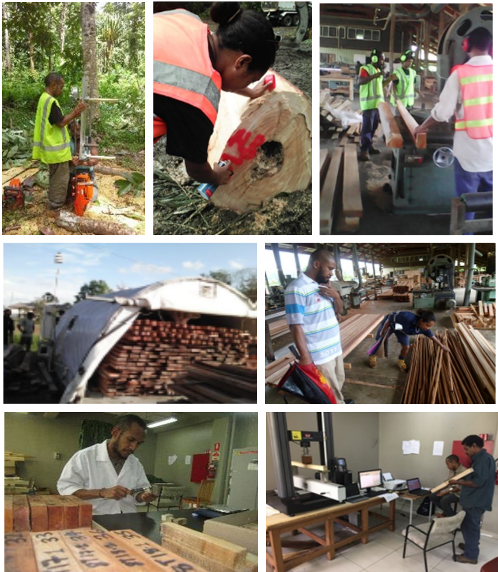
Figure 1. The process of samples preparation from harvesting to testing.
