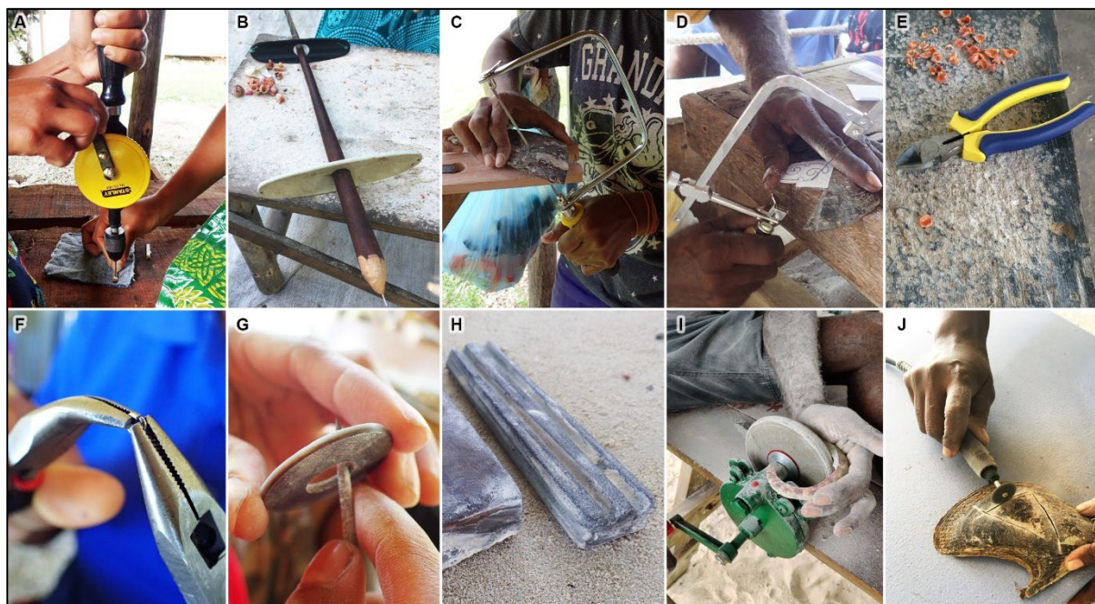
Tools that were used for shellcraft in PNG: (A) mechanical hand drill, (B) pump drill, (C) coping saw, (D) jewellery saw, (E) cutter pliers, (F) jewellery pliers, (G) needle file, (H) stone file, (I) grinder, and (J) electric rotary.
