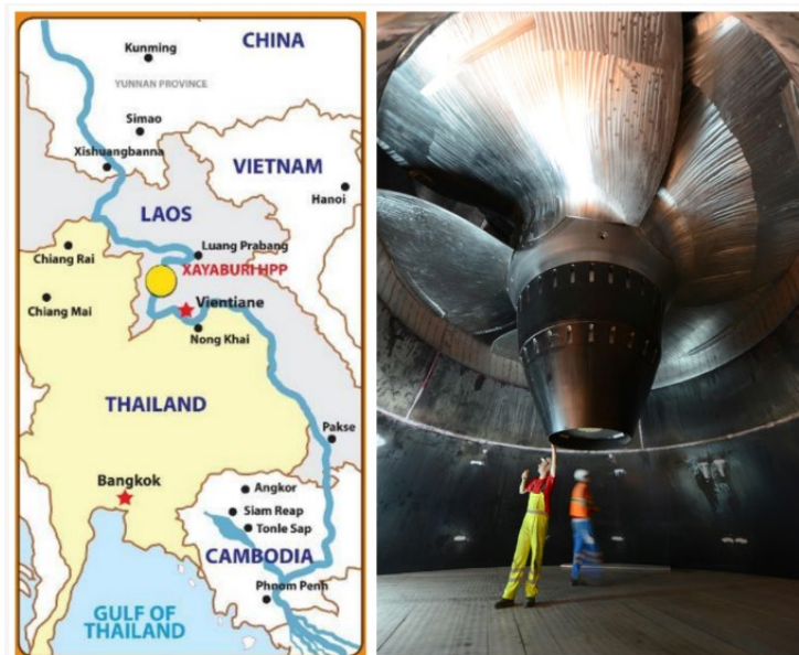
Figure 8. The location of the Xayaburi Hydroelectric Power Plant on the Mekong River in the northern Lao PDR (left), and the Kaplan-type runner tested (not to scale) (right) (source: Romero-Gomez et al. (2024)).
