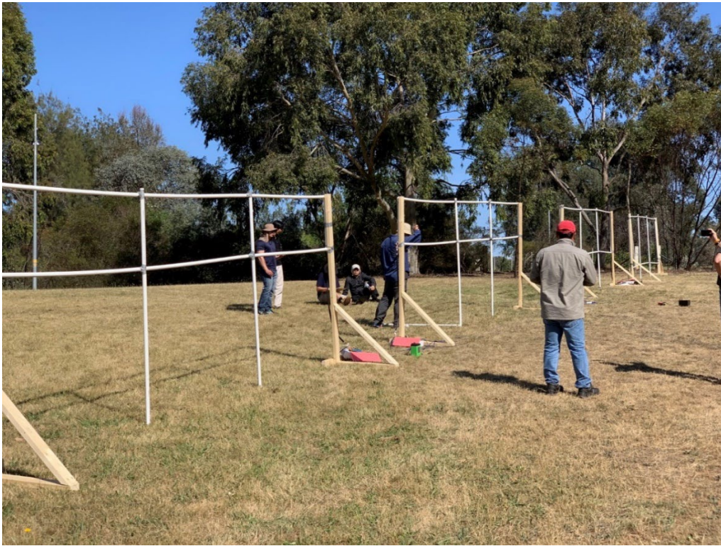
Figure A2.2. FIS/2017/017 team members conducting the antenna design experiments at CSU (Albury) in November 2018. This was the test of the four antennas, 1 x 6 m by 1.5 m; 1 x 6 m by 1.0 m; 1 x 6 m by 0.6 m; 1 x 6 m by 0.6 m) (source: Karl Pomorin). The white vertical supports for the antennas are not part of the actual antennas.
