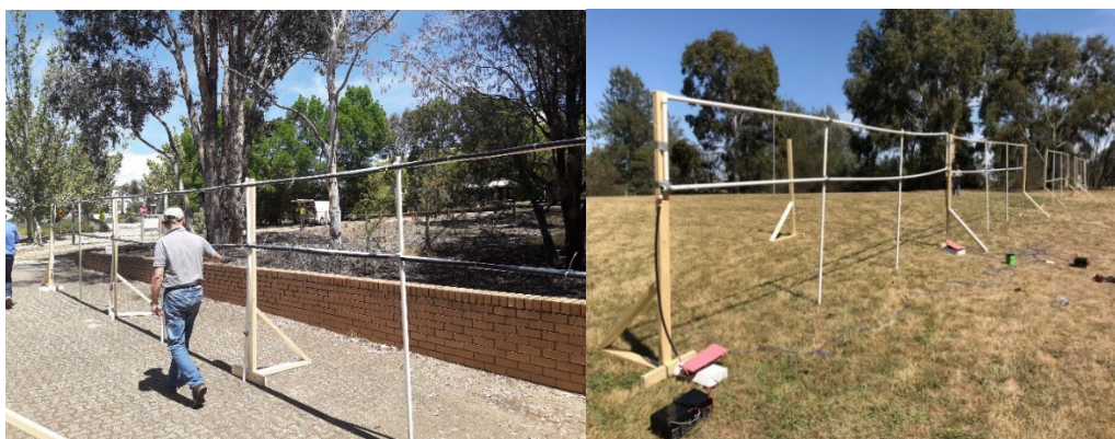
Figure 4. PIT antenna pre-installation testing at Charles Sturt University, Albury, NSW (source: Karl Pomorin)
