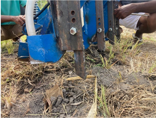
Figure 7.4: Hard-faced knife-points mounted in front of the tynes on the Thai seeder by Dom Bosco.
