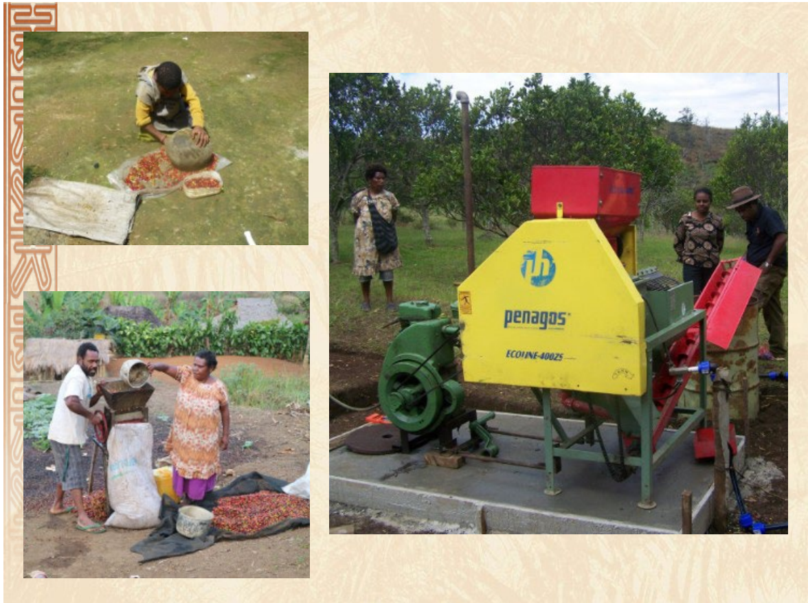
Plate 7.10: Changes in technology in coffee processing: stone pulper, hand pulper and demucilager.
