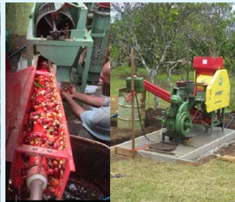
Using a demucilager to pulp cherry and remove the mucilage in one step.
