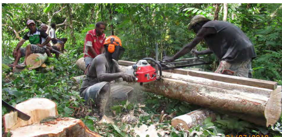
Figure 14-4: A sawmiller in Morobe Province producing rough-sawn lumber with a chainsaw milling attachment
