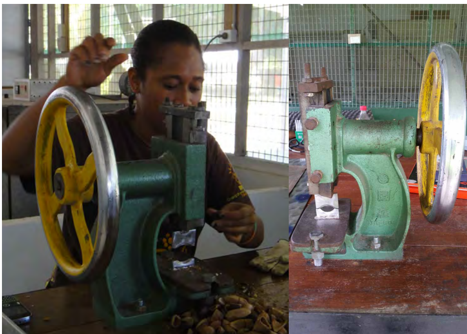
Figure 12-7: (Left) Small hand-operated benchtop crackers with (right) modified blades
