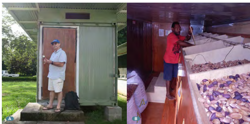
Figure 12-5: (Left) A large-scale nut-in-shell dryer constructed from a decommissioned refrigerated container and local materials. (Right) Inside the large-scale dryer.
