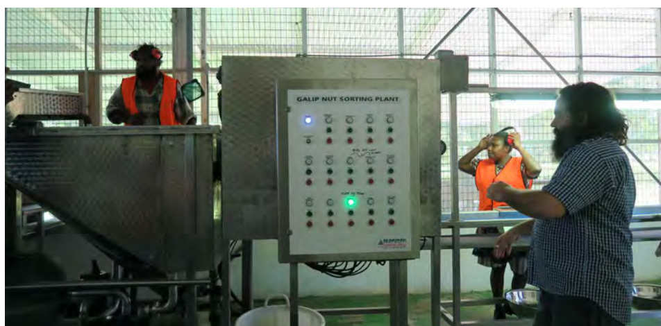
Figure 12-6: Mechanical cracker and the processing line commissioned to increase cracking capacity
