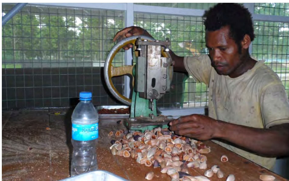
Figure 12-4: The dried, hard nut-in-shell is cracked to extract the edible kernel.
