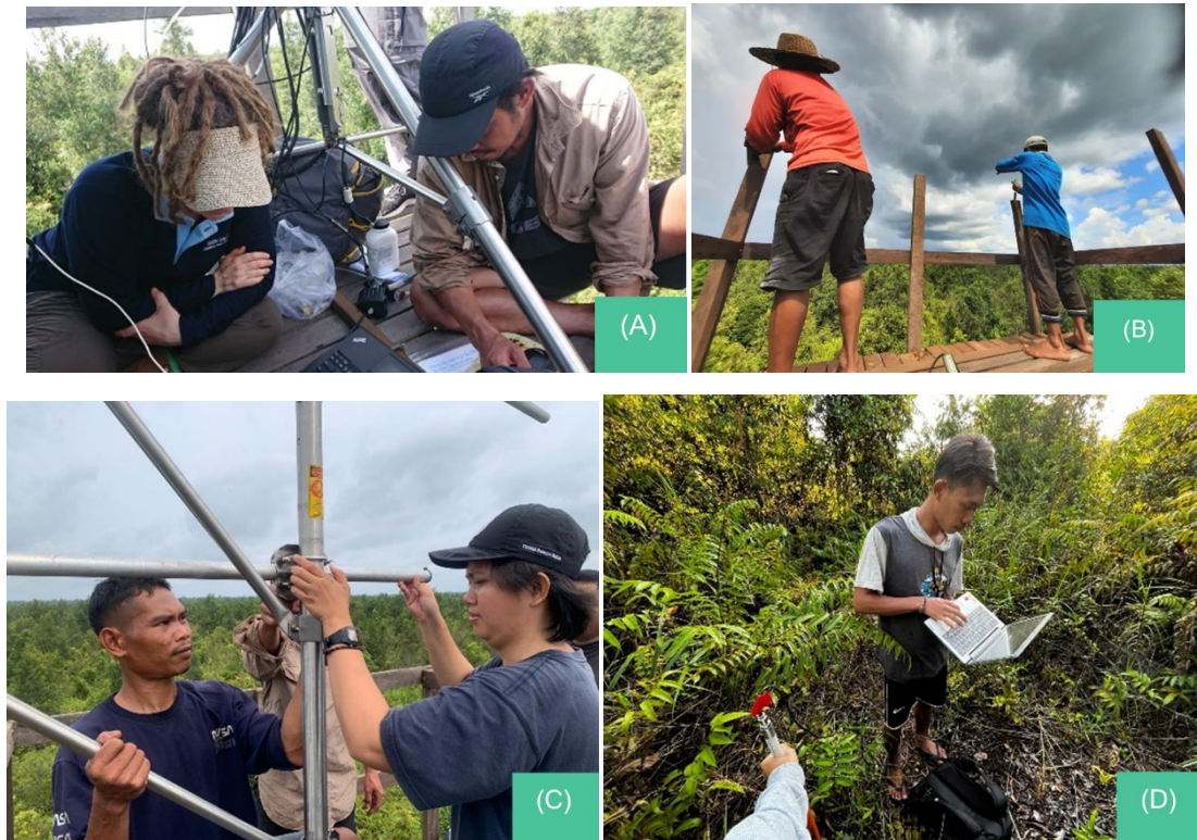
Figure 5. Equipment maintenance and reinstallation activities: (A) Checking the strength of CO 2 and H 2 O signals and replacing CO 2 scrubber bottles; (B) Raising the height of the Flux Tower; (C) Reinstallation of Flux equipment; (D) Repairing the automatic ground water logger.
