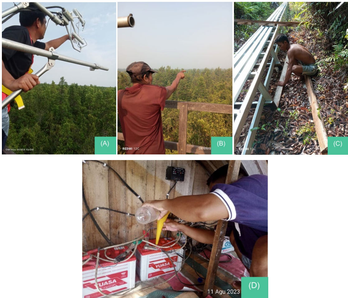
Figure 3. Daily monitoring in the Flux Tower area; (A) Routine cleaning of Flux Tower equipment: 3D Sonic-Anemometer; (B) Smoke and fire monitoring; (C) Walkway maintenance; (D) Refilling of Accu water.
