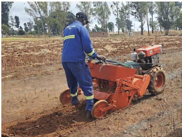
Figure 13 Prototype Bed planter fabricated at the Zimplow workshop in Bulawayo and tested at the Institute of Agricultural Engineering (IAE), Harare
