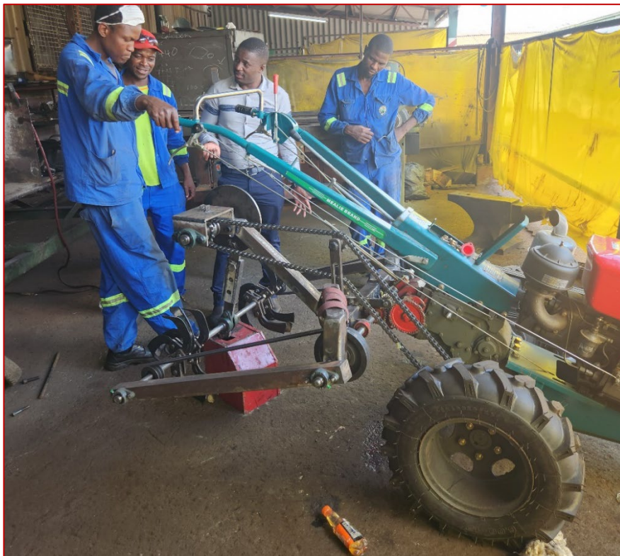
Figure 9 Fabrication of the Basin Digger Prototype 1 (two-wheel tractor operated) at the Zimplow factory in Bulawayo
