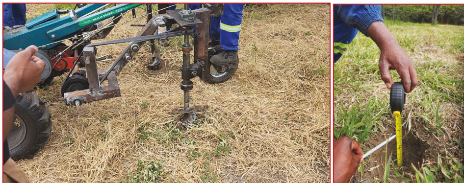
Figure 11 Field testing of the Basin Digger Prototype 2
