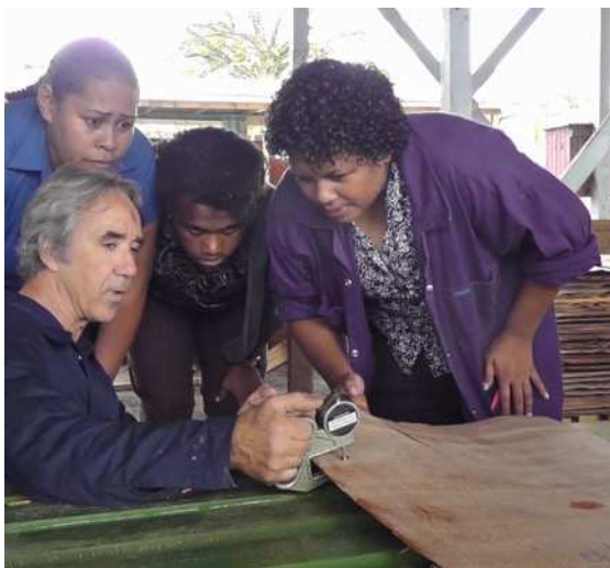
Figure 8: Accessing veneer thickness during Trial 3.
