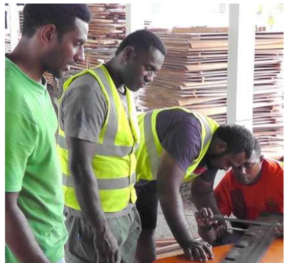
Figure 9: TUD staff replacing the veneer blade between peeling runs.
