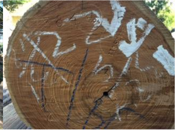
Marking of the log consists of tree number, cutting number, length of the log, volume and forest district.
