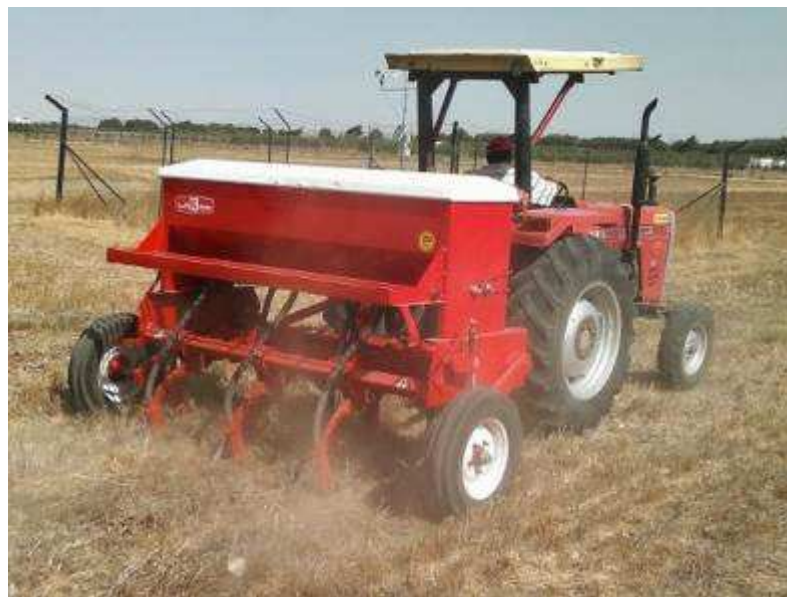
Fig. 6: Field testing of the Rama II ZT seeder produced in Jordan in September 2014.
