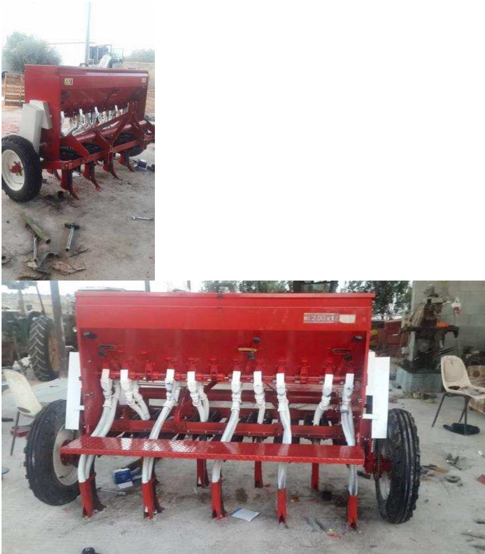
Fig. 9: The prototype compact ZT seeder developed in Jenin (Palestine), June 2015.
