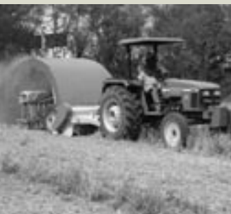
The 'Happy Seeder' sowing mung beans into wheat stubble
