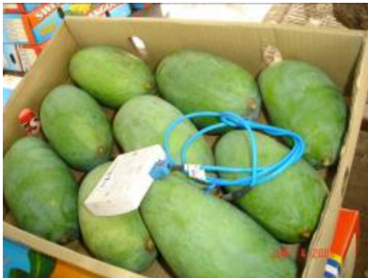
Fruit Box with Data Logger at Orchard
