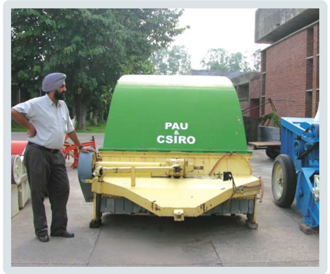
Dr Sidhu with a Happy Seeder, to be towed by a tractor.
