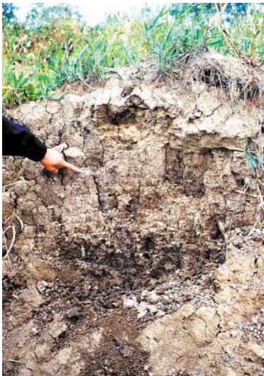
Figure 5. Sodicty subsoil formation. (Note that root development is restricted to the A1 horizon because roots find it difficult to penetrate the prismatic Bt horizon.)
