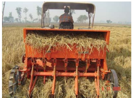
Figure 4. Happy Seeder for seeding into loose residues
