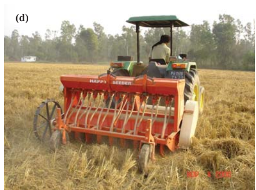
Figures 8a–d. The Turbo Happy Seeder showing: a) sowing with full cut in November 2005, b) establishment of wheat sown in November 2005, c) excellent crop in farmers' field sown in November 2005, d) sowing wheat in rice residues with partial cutting of the standing stubble
