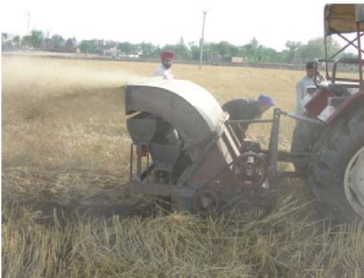
Figure 5. The Combo Happy Seeder sowing into wheat straw in May 2004 with full cutting
