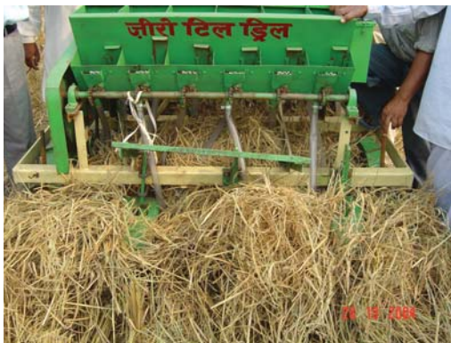
Figure 3. Star wheel / punch planter for seeding into loose residues
