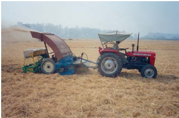
Figure 1. The first Mark 1 Happy Seeder with zero-till drill, powered by a 35 hp Massey Ferguson tractor, sowing on the flat in October 2002
