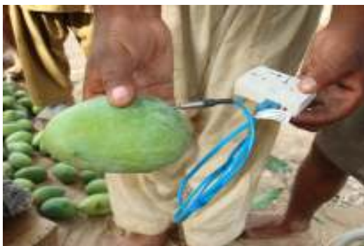
Data logger inserted in fruit for temperature monitoring
