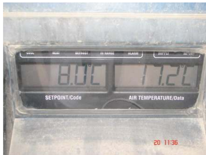
Set point of temperature and air temperature in a reefer container
