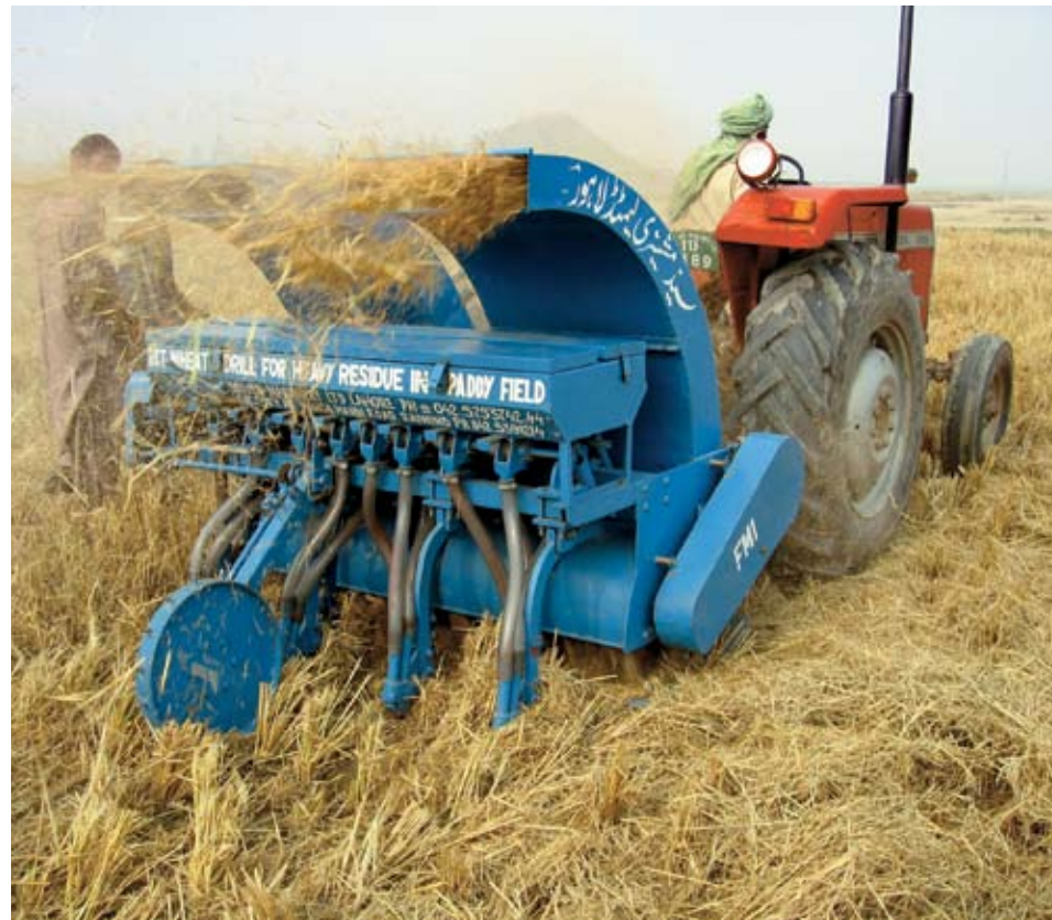
A seeder to allow planting of wheat into rice-straw stubble, similar to that now being trialled for raised beds.
