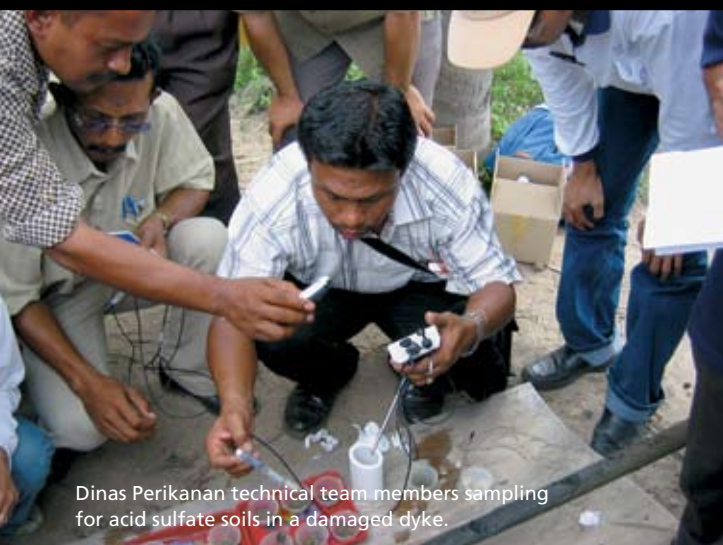
Dinas Perikanan staff measuring the pH of soil before and after oxidation to determine the acid-generating capacity of the soils.
