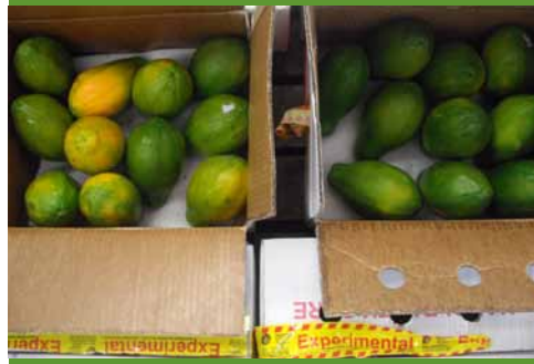
Preliminary observations in the carton performance trial indicate that papaya in the cartons with holes (right) did not ripen in transit, while those in the standard cartons (left) did.
