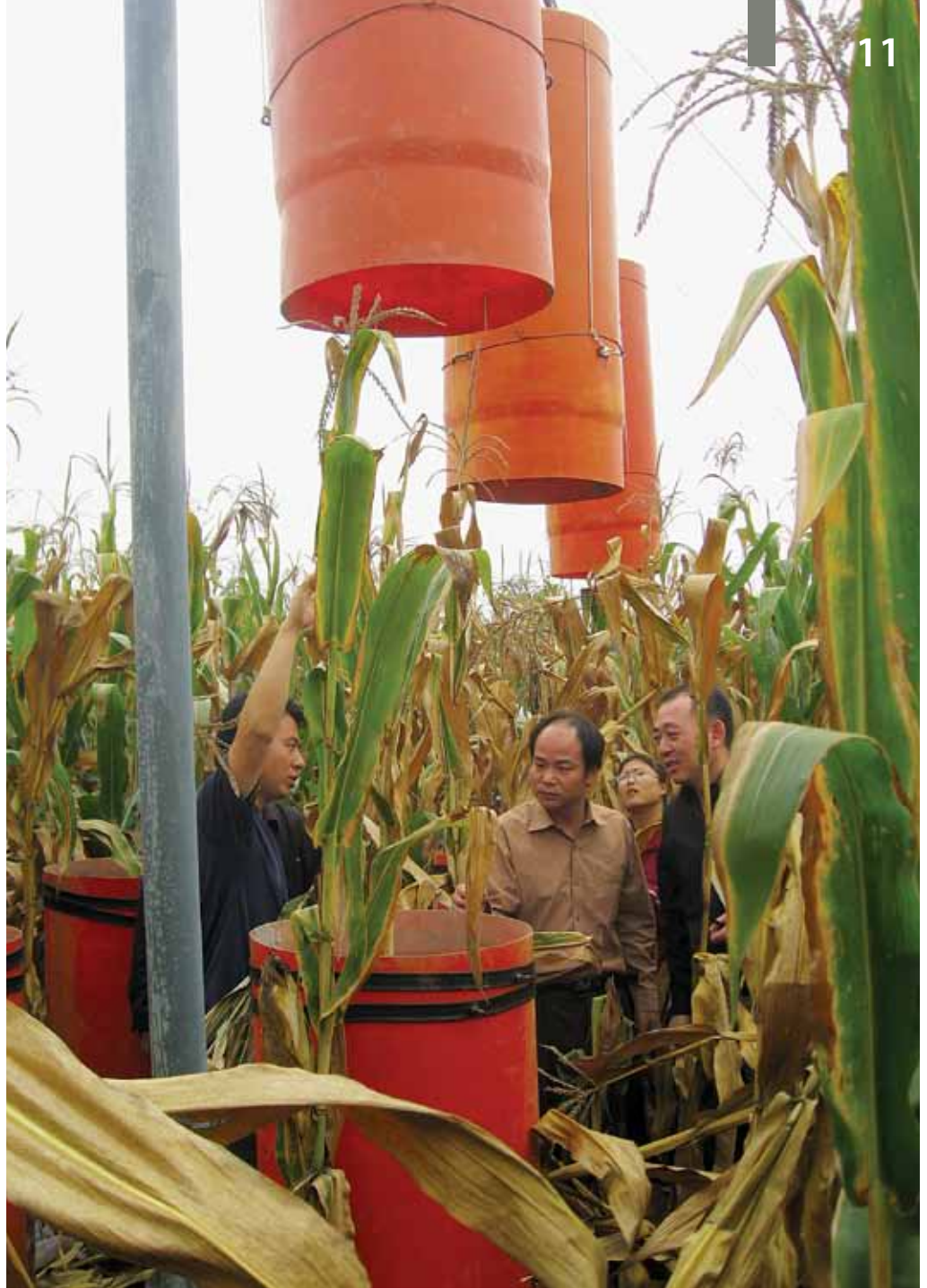
Dr Lin Yuntong and Dr Wan Yunfan with project leader Dr Deli Chen inspecting manual open-top chambers in a maize field.
